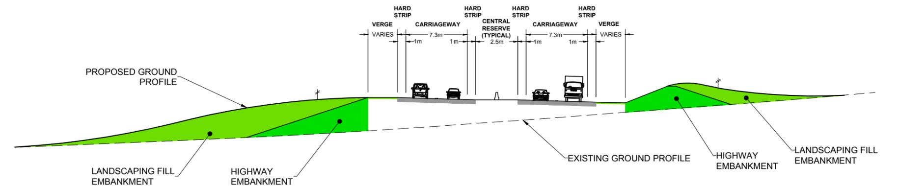
Figure 5.5: Typical cross section
