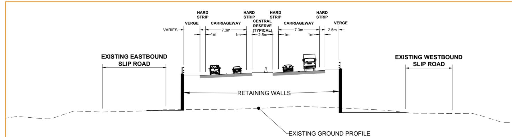
44 **Figure 5.46: The cross-section above illustrates how the flyover would be constructed between the existing approaches to Countess roundabout which would then become the slip road connections between the new A303 and the A345.**
